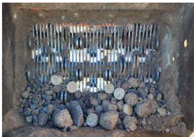
b) Multiple replica PMN-4 AP mines left over inside the same bucket after screening
