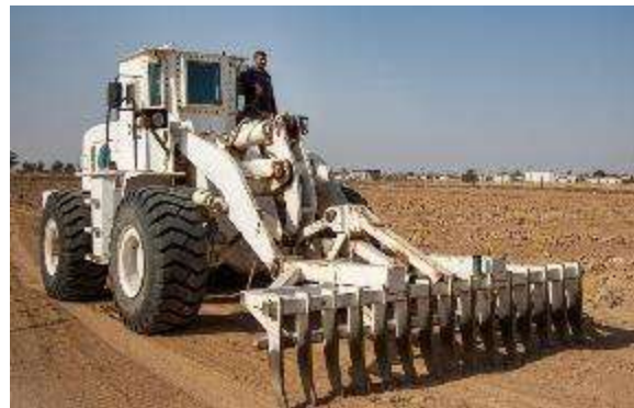
b) Wheel loaders with front mounted scarifier attachment – typically used for technical survey searching for IEDs
