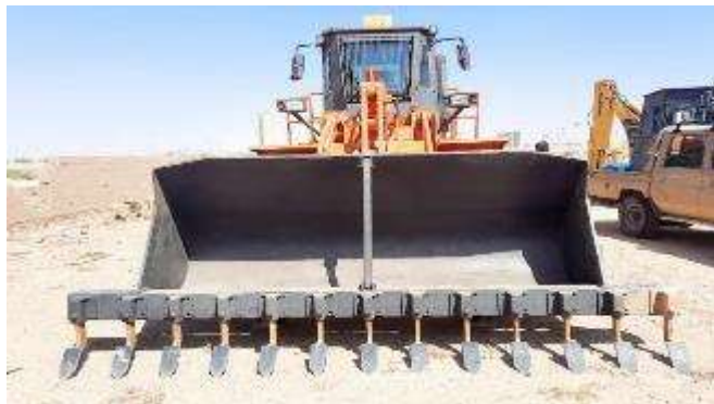
a) Wheel loaders with front mounted rake attachment – typically used for technical survey searching for IEDs
