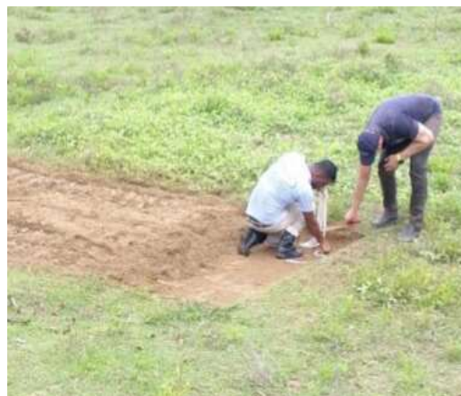
b) Measuring and recording penetration depth during safe area testing
