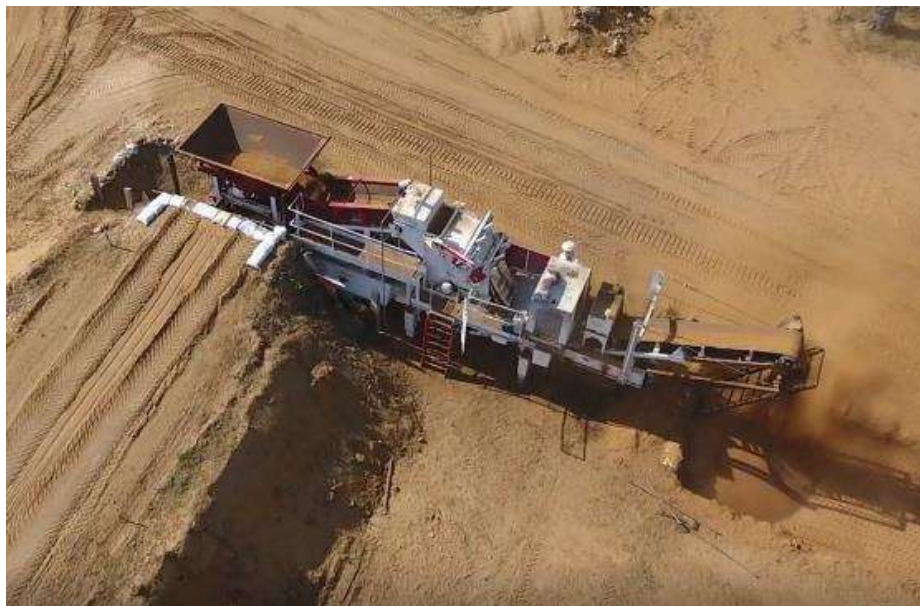
Figure 1 – Example of an impact crusher unit used to destroy plastic-bodied anti-personnel blast mines – The HALO Trust
