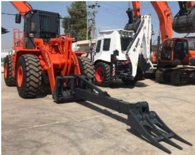
a) Wheel loader with extended rake attachment
