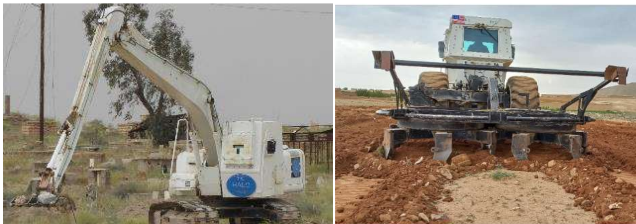
a) Tracked excavator with rake attachment – typically used for technical survey or clearance of IEDs b) Rotary mine comb (RMC) attached to a tractor – typically used for clearance of minimum metal AV mines
