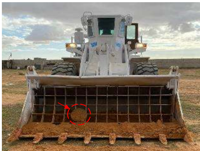
a) Wheel loader with screening system fitted to the bucket and AV mine shown inside the bucket
