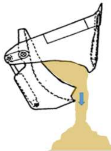
b) Diagram showing a multi-purpose (4 in 1) bucket from the side
