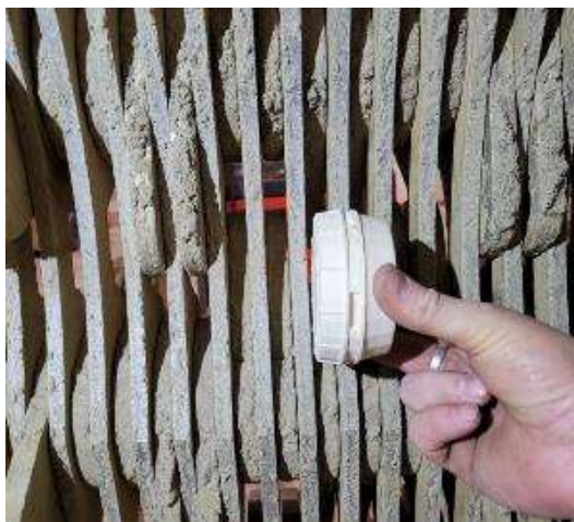
a) Replica PMN-4 AP mine unable to pass through a screening bucket configured to 16 mm spacing
